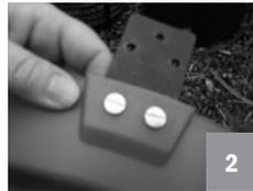
Photo 3: Attach the lid to the outer Cone without the black liner in place. Use three screws (part C) to attach the lid hinge (part A) to the outer Cone. There may be a small rectangular piece of ridged plastic (part D), which can be used inside the outer Cone as reinforcement. The screws are sharp and self-drilling.
