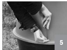
Photo 6: Set the outer Cone and liner on top of the black basket. Attach the Cone and liner to the basket using screws (part C). The screws are self-drilling and with a little pressure, will drill their own holes through the plastic. Use six screws to attach the basket to the outer Cone and liner.
